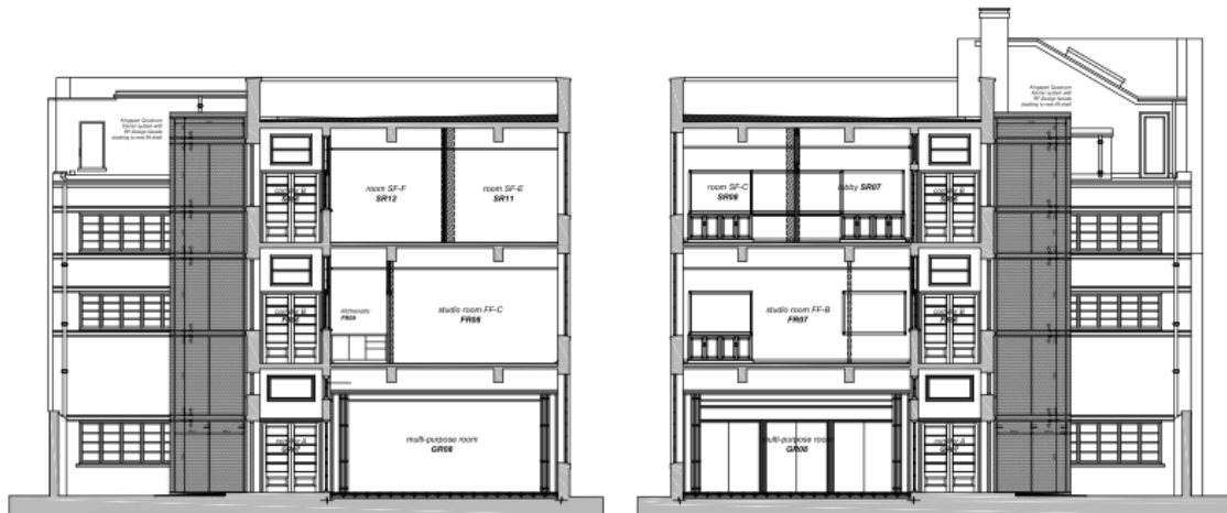
SECTION B-B / LIFT ELEVATION 1:50
